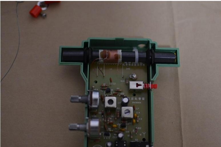
[ ] Finally, connect the telescope antenna W by a Philip screw driver. Place the lock washer in between the solder layer of the PCB and the telescope antenna. Note that don't scratch the cover paint on the antenna, or it will be easier to short circuit with the PCB.
