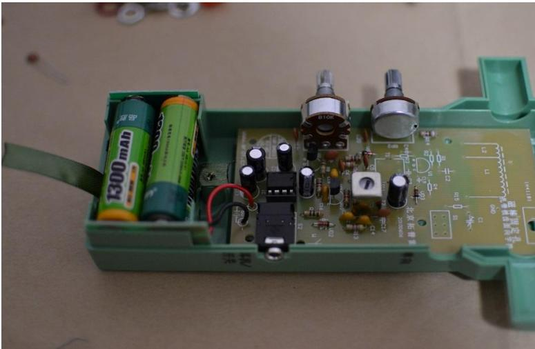
[ ] Now you will need to use a SSB or CW receiver to align the oscillator frequency coverage. In my example, I connect a dummy load to the transceiver, and put the dummy load near the kit, and adjust the frequency near 3.55-MHz in CW mode. Turn RP2 to the middle, where you can feel a stop, and adjust shielded coil T2, so you can hear a tone in the transceiver. You can turn RP2 to the two ends to make sure the frequency coverage is a bit wider than 3.5~3.6-MHz. I don't want to
