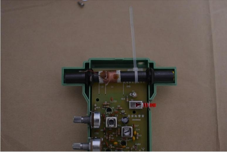
[ ] Cut the extra strip. Solder 3 tinned ends of the coils on the magnetic rod to the board. See the PCB marking to connect the right windings (less turns on the left).
